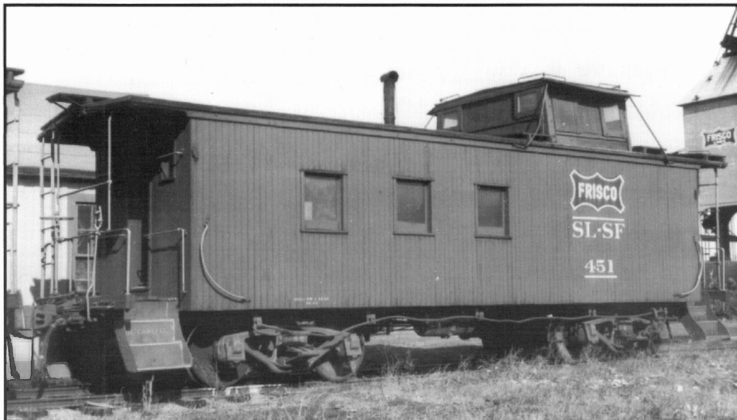
Frisco standard design steel underframe caboose 451, shown here in service at Ft. Smith, AR, December 28, 1952. Photo from the collection of John C. LaRue.
