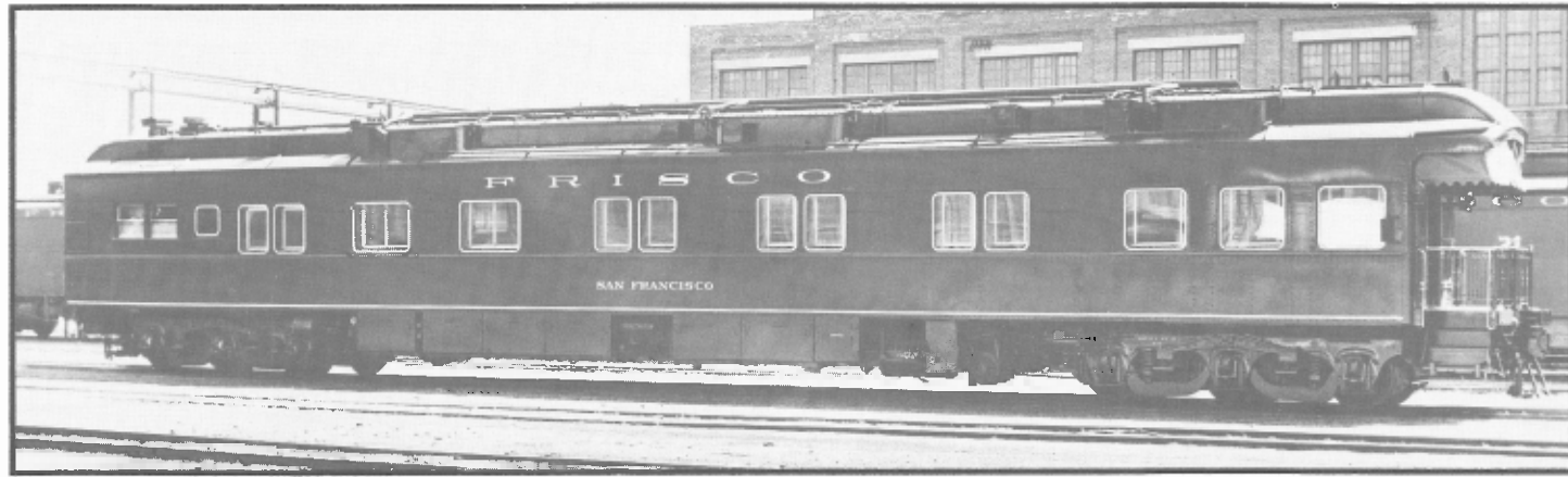
Left side view, Frisco Business Car San Francisco, with monitor roof design, West Springfield Coach Shops, April 17, 1952 Frisco photo
