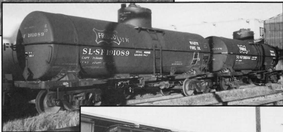
Frisco company service tank cars, series 191000-191129, were built by American Car & Foundry in July 1949. They were 36' units with a capacity of 10,000 gals. and were used for transporting diesel fuel. Frisco Folk Wayne Porter found 191089 & 191006 still in service at Lincoln, NE, November 19, 1993.
