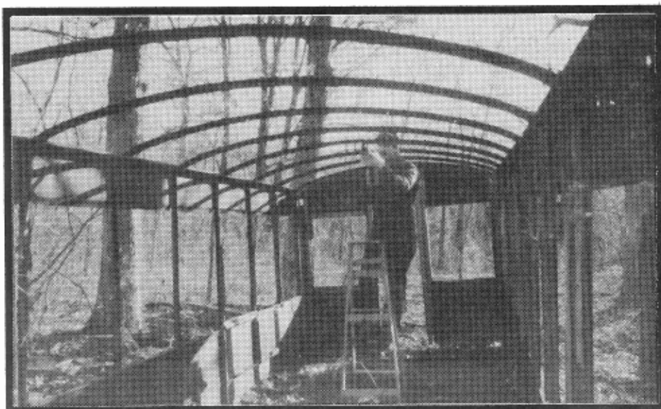
Frisco Folk Matt Collins begins process of cutting car into two sections. The "path" into the woods where the car was located was too narrow to move it in one piece.
